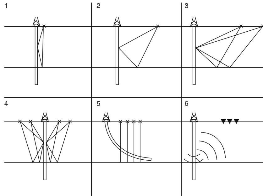
**Vertical Seismic Profiling, Figure 1** Common acquisition geometries for vertical seismic profiling (VSP): (1) zero-offset VSP (ZVSP), (2) offset VSP, (3) multi-offset VSP, (4) walk-away VSP, (5) walk-above VSP, and (6) drill-bit SWD (seismic while drilling) VSP.
