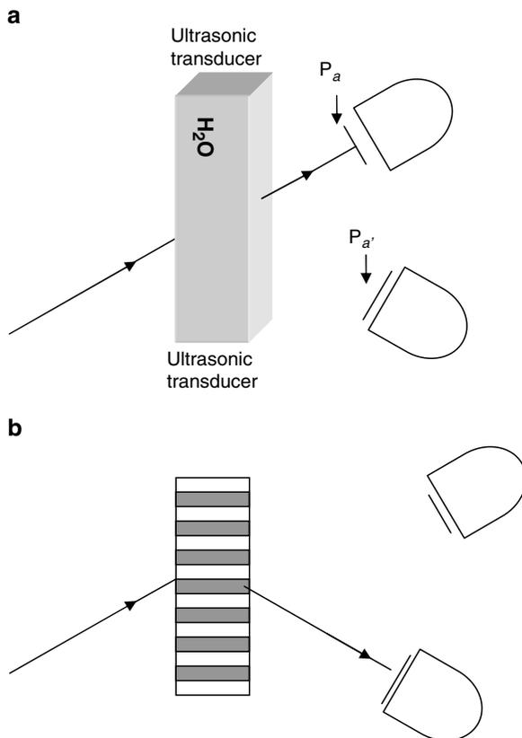
**Fig. 1** Schema of switching devices in Aspect experiment.  $P_a$  ( $P_{a'}$ ) are polarisers with transmission axis  $a$  (**a**). When a photon arrives at time on ultrasonic cycle when density of  $H_2O$  is constant, it is directed into  $P_a$ ; (**b**) if it arrives at a maximum of the standing wave, into  $P_{a'}$
