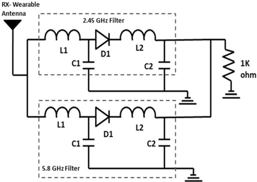
Fig. 3 Electrical circuit of rectenna
