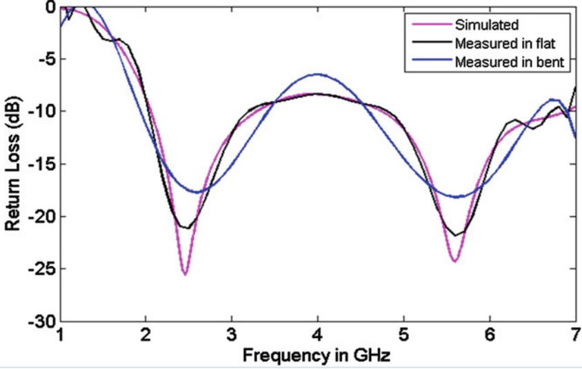
Fig. 4 Comparative return loss of the proposed antenna
