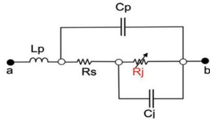
conversion is HSMS2850 with a low threshold voltage of 150 mV [12]. The input impedance of the diode is a dynamic variable dependent on input RF power, in order to understand that diode performance a mathematical model of the diode undergoes detail analysis with spice parameters given in Table 2.
