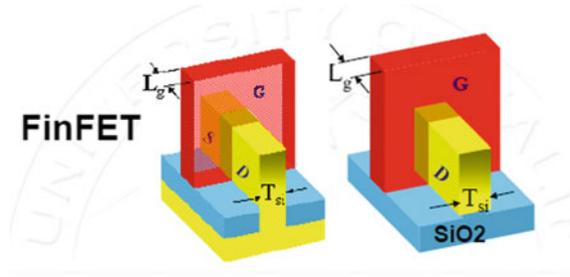
**Fig. 6** Fin on bulk and fin on SOI
