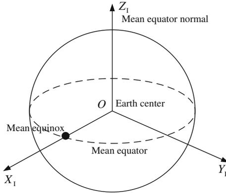
Fig. 2.7 J2000.0 Earth centered inertial coordinate system
