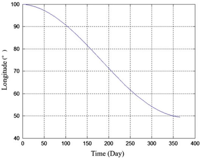
Fig. 2.2 Longitude drift of GEO satellite within a year
