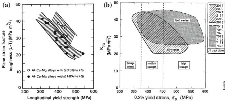
**Fig. 2.3** Plane-strain fracture toughness of **a** Al-Cu-Mg alloys with differing levels of iron and silicon [3]; **b** 2XXX and 7XXX alloys covering three strength regimes [7]. Note the general inverse relationship between strength and fracture toughness
