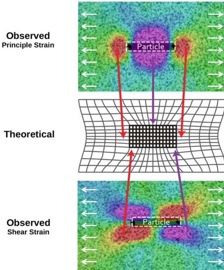
**Fig. 5** Comparison of observed strains (obtained from DIC) and a theoretical representation of the interaction between an embedded particle and a polymer matrix. Theoretical model adapted from Clyne (1989)
