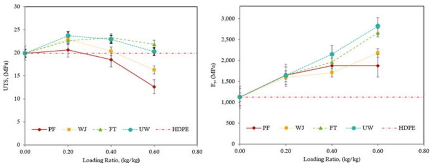
**Fig. 4** *Left* Ultimate tensile stress versus wood filler loading ratio; *PF* pine flour, *WJ* whole-tree juniper, *FT* forest thinning, *UW* urban wood, *HDPE* reference specimen with no filler (Karas 2010)
