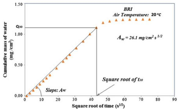
30 min method presented almost the same results. However, some building materials (*mcb30/70* and *mcb25/75* mortars) exhibit a slow initial water absorption rate and thus, the 30 min method estimates smaller values compared to the values given with the other two estimation methods. In Fig. 6, the capillarity rise kinetics, at 20 °C
