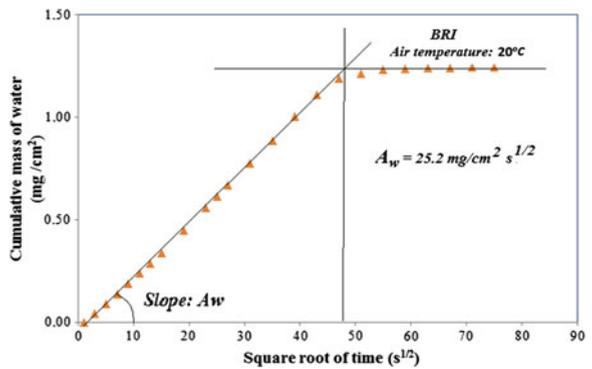
**Fig. 5** Determination of water absorption coefficient due to capillarity according to UNI 10859
