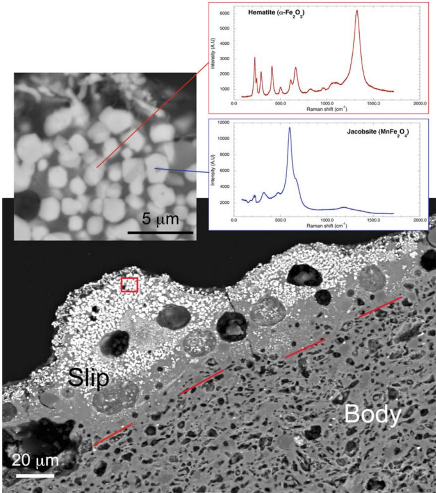
**Fig. 3** Cross-section of a black decor of a Cucuteni ceramic containing both hematite and jacobsite crystals
