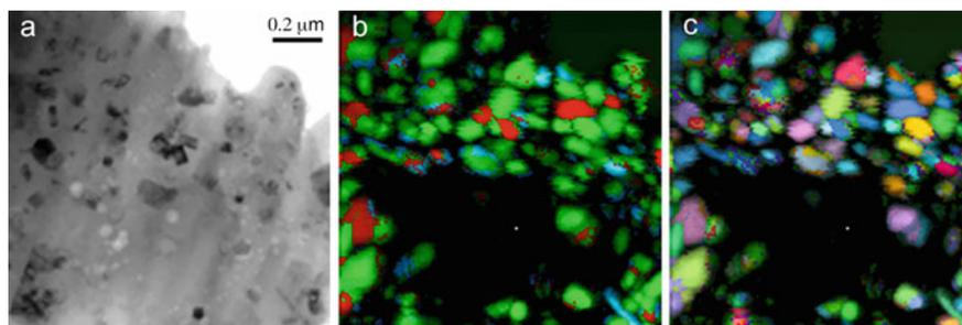
**Fig. 10** Gallic terra sigillata coating observed in TEM. **a** Bright field image, ASTAR high resolution phase **(b)** and orientation **(c)**. The coating **b** consists of hematite (in red), corundum (in green) and spinel (in blue) crystals in a glass matrix. There is no particular orientation of crystals **(c)**
