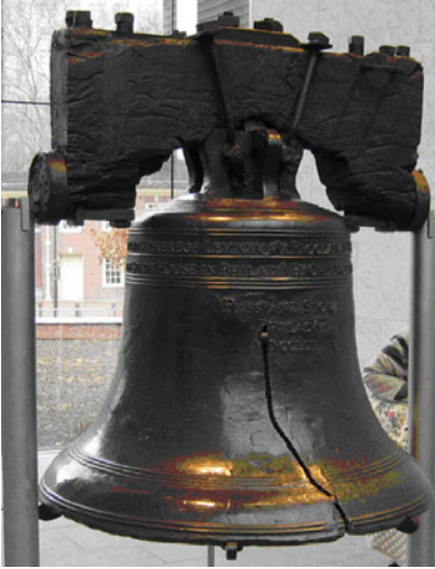
Fig. 2.2 Macroscopic brittle fracture of the Liberty Bell, Philadelphia 1752
