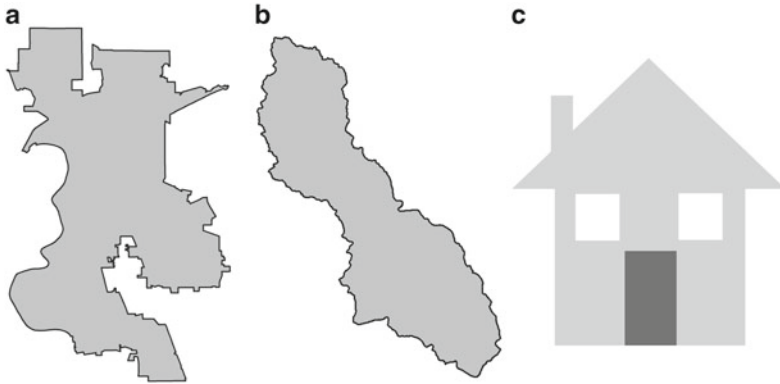
Fig. 2.5 Defining system boundaries. The budgetary approach can be applied to any system but the boundary of the system must be delineated so that what is in and what is out can be determined. Three different system boundaries are shown – the municipal boundary of Sacramento, California (panel a), the watershed boundary for the Gwynns Falls in Baltimore, Maryland (panel b), and a household (panel c). A specific research question determines which boundary is appropriate. Published with kind permission of © Mary L. Cadenasso, 2013. All Rights Reserved
