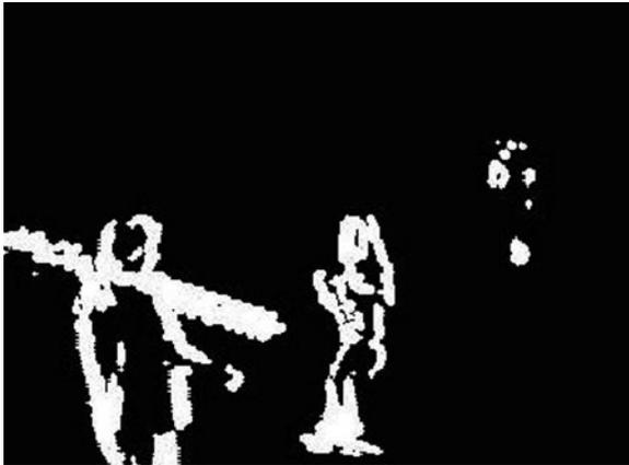
Fig. 2.16 Blob detection by optical flow
