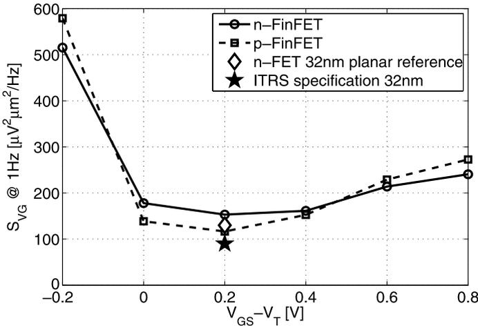
**Fig. 2.8** Comparison of measured spectral noise density of FinFET and planar devices for varying gate overdrive at 1 Hz
