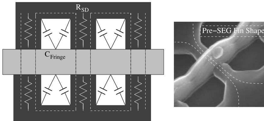
**Fig. 2.4** Schematic view and SEM picture of FinFET before and after SEG including parasitics
