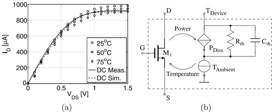
**Fig. 2.15** Comparison of pulsed and DC  $I_D$ - $V_{DS}$  measurements/simulation (a) and equivalent circuit model for self heating (b)
