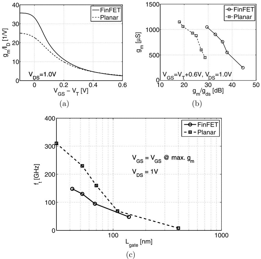
**Fig. 2.6** Measured efficiency  $g_m/I_D$  of n-type planar and FinFET device with 90 nm gate length (a),  $g_m$  vs  $g_m/g_{ds}$  trade-off (b) and transit frequency  $f_t$  (c) of planar and FinFET devices for varying  $L_{gate}$
