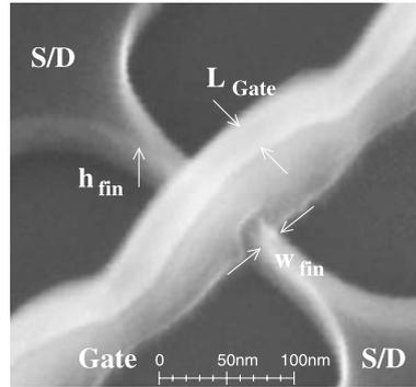
**Fig. 2.1** FinFET process flow and SEM picture of single fin device after gate patterning
