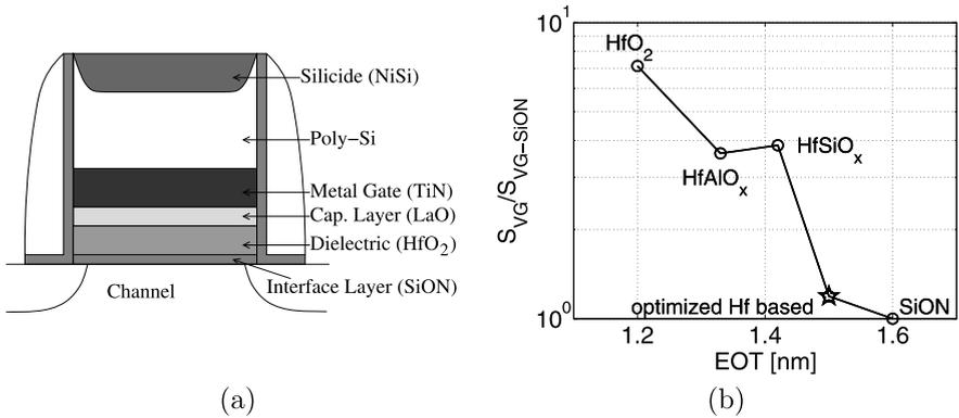
**Fig. 2.7** Schematic cross-section of high- $k$ /metal gate stack with exemplary materials (a) and relative flicker noise vs EOT trade-off for different dielectric materials (b) [65]
