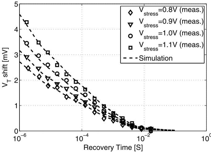
Fig. 2.14 Measured and simulated recovery of  $V_T$  shift for varying gate pulse height and measurement delay
