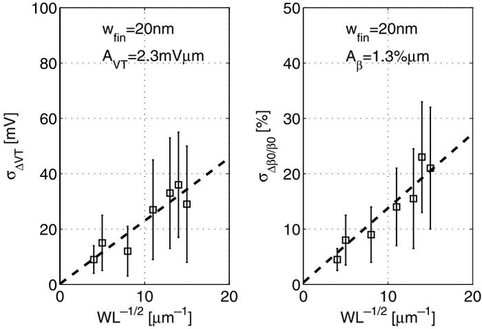
**Fig. 2.10** Pelgrom plots of n-type FinFET with 20 nm fin width for  $V_T$  and  $\beta$  matching
