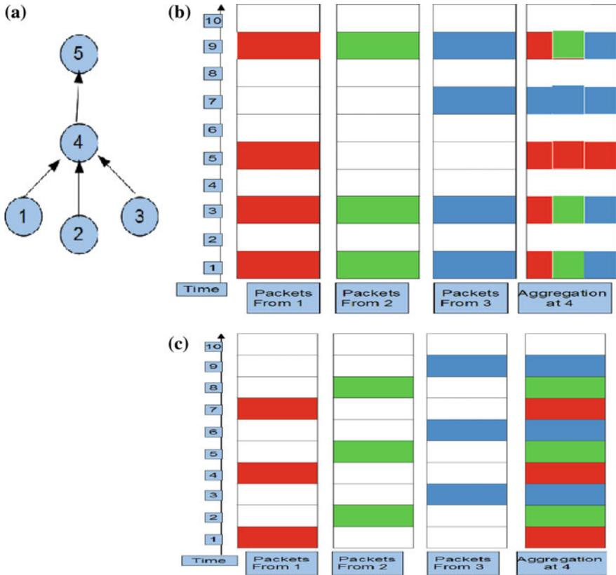
Fig. 1 Case 1: an example of data aggregation constraint
