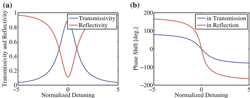
**Fig. 2.3 Optical cavity.** These show the reflected and transmitted fields as a function of detuning normalized by the cavity decay rate. **a** The (power) reflectivity and transmissivity are shown. **b** The phase shifts in reflection and transmission are shown
