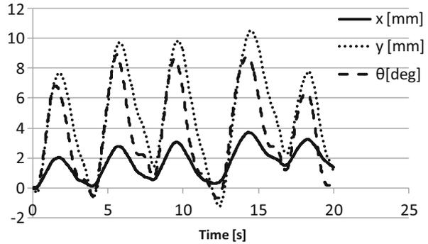
**Fig. 2.8** Tracking error (detected relative position of the probe against the image)
