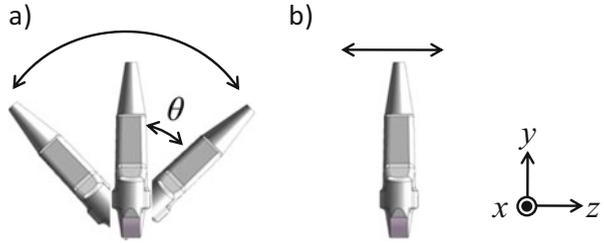
initial scanning  $LN$  is set as  $\pm 10^\circ$ . In this case, the scanning distance at the depth 50 mm (the center of the image) is 17.5 mm.
