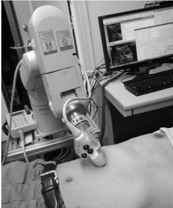
Fig. 2.5 Experimental setup of the liver tracking
