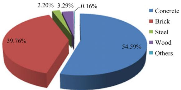
building waste is concrete and bricks, together with a little amount of steel and wood, all of them can be recycled. Considering the fact that the disaster area is faced with many challenges such as shortage of resources after the earthquake, it is quite important to get information on the amount and types of the building waste as well as the corresponding reclaiming methods.
