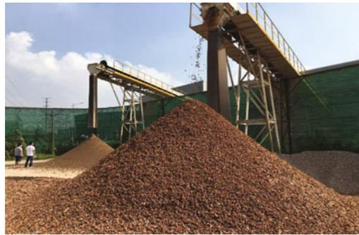
(a) The production line of recycled aggregates
