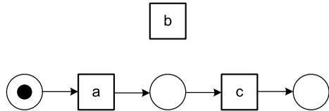
**Fig. 6.11** WF-net  $N'_7$  having a so-called “short-loop” of length one
