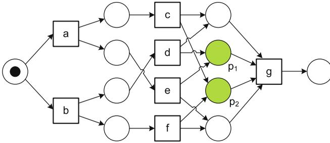
**Fig. 6.9** WF-net  $N_6$  derived from  $L_6 = [\langle a, c, e, g \rangle^2, \langle a, e, c, g \rangle^3, \langle b, d, f, g \rangle^2, \langle b, f, d, g \rangle^4]$ . The two highlighted places are redundant, i.e., removing them will simplify the model without changing its behavior
