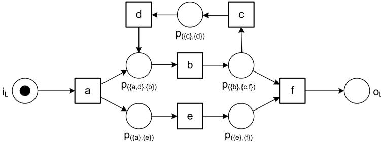
**Fig. 6.8** WF-net  $N_5$  derived from  $L_5 = [\langle a, b, e, f \rangle^2, \langle a, b, e, c, d, b, f \rangle^3, \langle a, b, c, e, d, b, f \rangle^2, \langle a, b, c, d, e, b, f \rangle^4, \langle a, e, b, c, d, b, f \rangle^3]$
