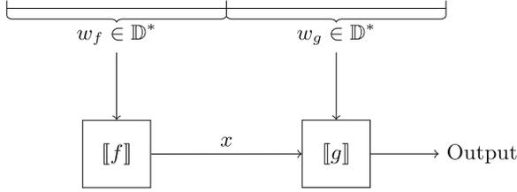
**Fig. 2.** The split combinator,  $\mathit{split}(f \ [x] \ g)$ , divides the input data string  $w$  into two parts,  $w = w_f w_g$ , applies  $f$  to  $w_f$  and  $g$  to  $w_g$ , and substitutes the result of  $f$  into the parameter  $x$  of the term generated by  $g$ . The expression  $\mathit{split}(f \ \langle x \rangle \ g)$  is similar except for the direction of the  $f$ - $g$  data flow.
