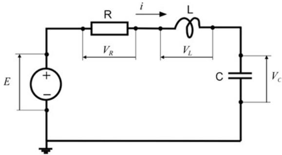
voltage source generating an electromotive force (e.m.f.)  $V_S$ , a resistor  $R$ , an inductor  $L$ , and a capacitor  $C$ . The polarities of the voltage drop across the electrical components are also shown, as well as the assumed direction of the current flow. We can develop a bond graph model using an approach similar to the mechanical system analysed previously.
