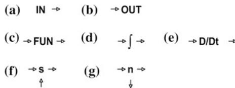
**Fig. 2.10** Basic block diagram components: **a** input, **b** output, **c** function, **d** integrator, **e** differentiator, **f** summator, **g** node
