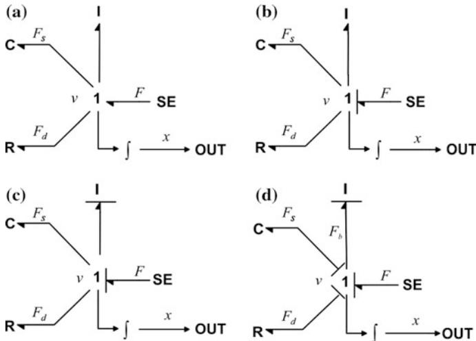
Fig. 2.30 Illustration of the causality assignment procedure
