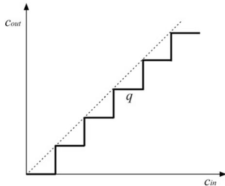
**Fig. 2.13** Model of A/D converter
