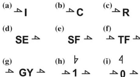
**Fig. 2.6** Elementary components: **a** inertial, **b** capacitive, **c** resistive, **d** source effort, **e** source flow, **f** transformer, **g** gytrator, **h** effort junction, **i** flow junction
