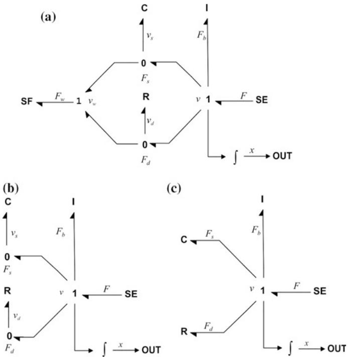
Fig. 2.16 Simplification of the bond graph of Fig. 2.15
