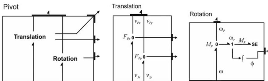
Fig. 2.24 Model of the see-saw pivot
