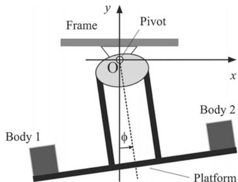
This problem is more complicated than those presented previously, as it consists of three interconnected bodies moving in the vertical plane. The model could be developed easily by treating the system as a physical pendulum. Instead, we consider it as a multi-body system and demonstrate how the model can be developed systematically by decomposition.
