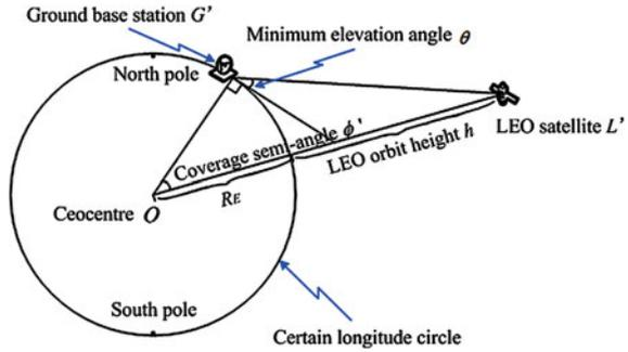
**Fig. 2.9** Schematic diagram of the ICO constellation
