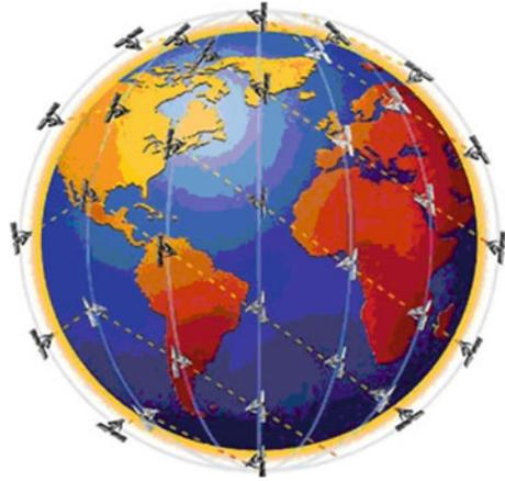
**Fig. 2.5** Top view of an inclined orbit constellation
