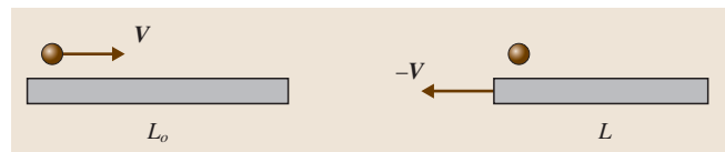
Fig. 1.4 Relative motion bar-particle in the proper frames of the bar ( left ) and the particle ( right )
