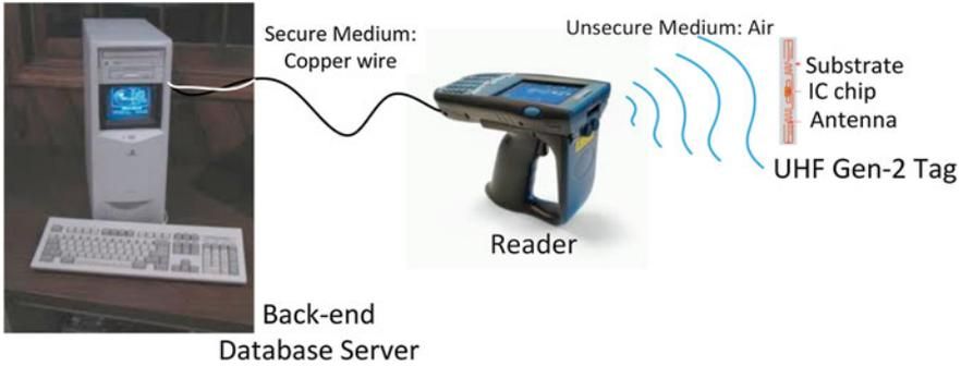
**Fig. 1.** A typical UHF RFID tag reading scenario
