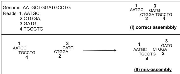
**Fig. 1 Genome misassembly by greedy algorithm.** (I) A small genome is to be assembled from four reads, labeled 1, 2, 3, and 4. The correct assembly is 1–2–3–4. (II) The greedy algorithm assembles 1 and 4 first, since they have the best overlap, of three nucleotides, and then 2 and 3 are assembled. As a result, the misassembled genome 1–4–2–3 is obtained
