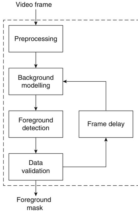
pre-processing can be performed to reduce camera and environmental noise such as rain and snow. Frame size reduction can also be performed to reduce the data processing rate. Background modelling is then performed to use the new video frame to calculate and update the background model. Various models can be used. These range from simple frame differencing to more sophisticated models using mixture of Gaussians.
