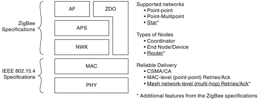
**Fig. 2.16** ZigBee layers and specifications
