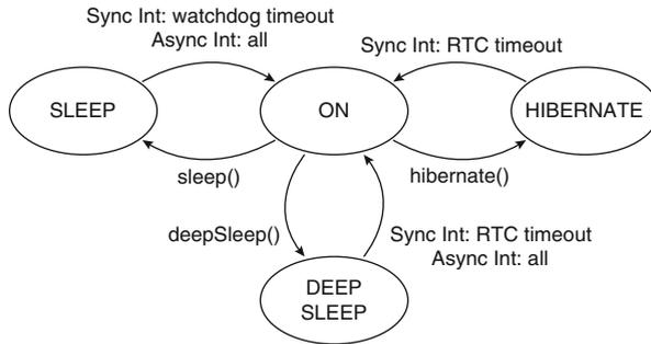
Fig. 2.7 State diagram for Wasmote operational modes
