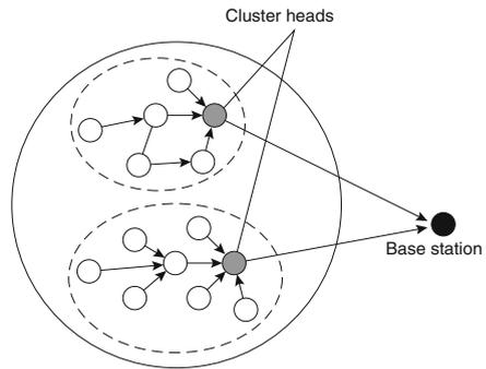
**Fig. 2.6** Hierarchical multi-tier multi-hop network architecture
