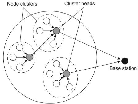
**Fig. 2.5** Hierarchical single-tier multi-hop network architecture
