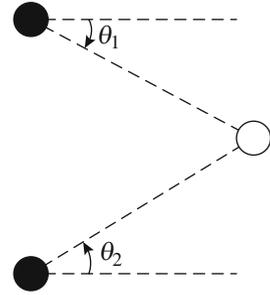
An AOA-based positioning technique involves measuring angles of the target node seen by reference nodes (triangulation) which is done by means of antenna arrays. To determine the location of a node in a two-dimensional (2D) space, it is sufficient to measure the angles of the straight lines that connect the node with the two reference nodes as shown in Fig. 2.18.
