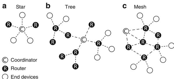
**Fig. 2.17** ZigBee network topologies
