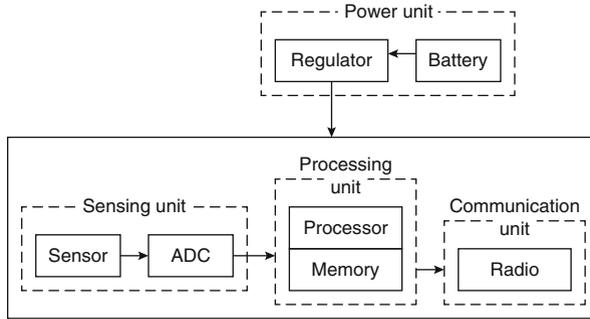
**Fig. 2.8** Components of a typical WSN node
