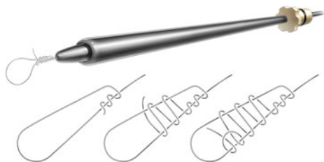
Fig. 2.21 Principle of the pretied knots
