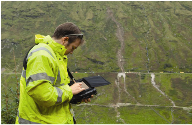
Fig. 2 BGS landslide survey using a ruggedised tablet PC with BGS•SIGMAmobile
