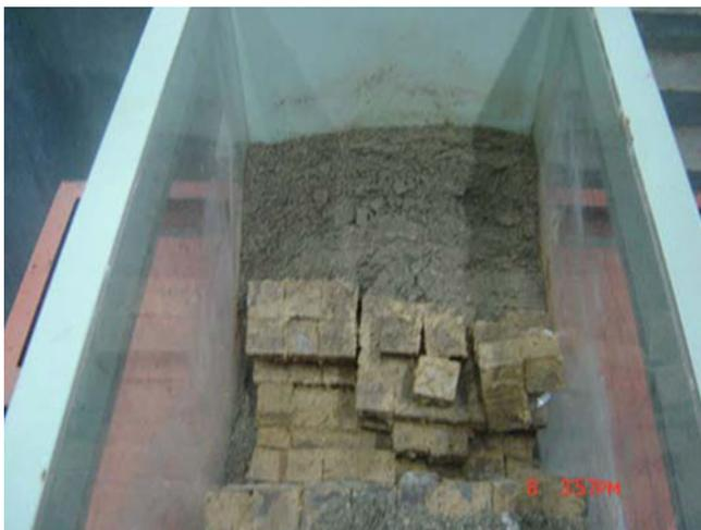
**Picture 3** Third level sliding face destabilization occurs on the consequent slope
