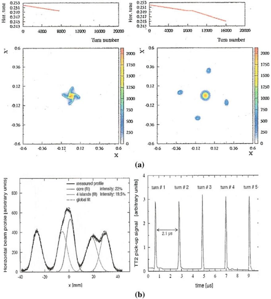
**Fig. 2.9** **a** New multiturn extraction for high intensities beam splitting on stable phase space Islands, approaching a 4th order resonance. **b** New multiturn extraction for high intensities. *Left:* Split beam in the PS, as seen on a beam profile monitor. *Right:* Beam signal in the transfer channel beyond the PS
