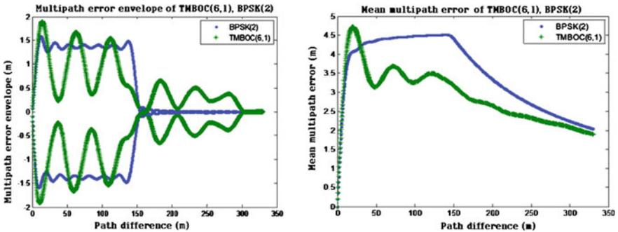
Fig. 8 Multipath error envelope (left), multipath error (right) of BPSK(2) and TMBOC
