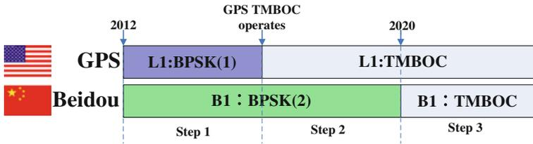
**Fig. 1** Phases of interoperability between Beidou and GPS
