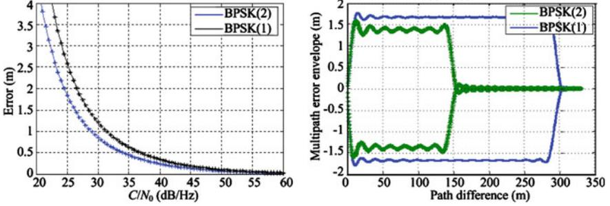
**Fig. 2** Tracking error (*left*), multipath error (*right*) of BPSK(1) and BPSK(2)
