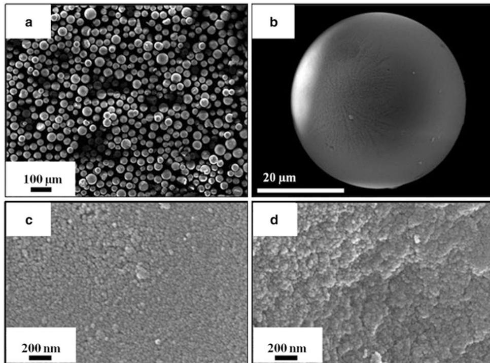
**Fig. 4** (a) Scanning electron micrograph (SEM) of the silica particles with an average size of 40  $\mu\text{m}$ . (b) SEM of a single silica sphere. (c) Field emission gun (FEG) SEM of a silica sphere external surface structure. (d) FEG SEM of a broken silica sphere
