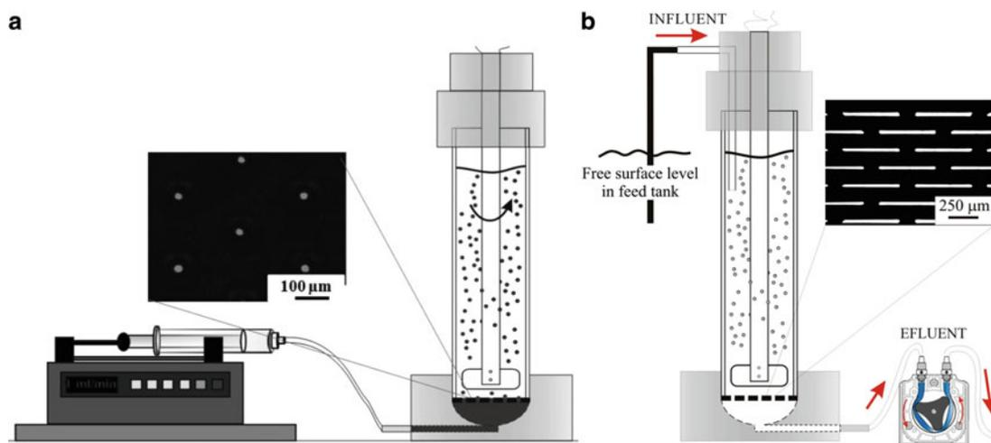
**Fig. 1** Schematic illustration of: (a) Dispersion Cell containing a paddle stirrer above a disk membrane with cylindrical 15 µm pores used for membrane emulsification and (b) microfiltration system with slotted pore membrane used for combined microfiltration/ion exchange experiments
