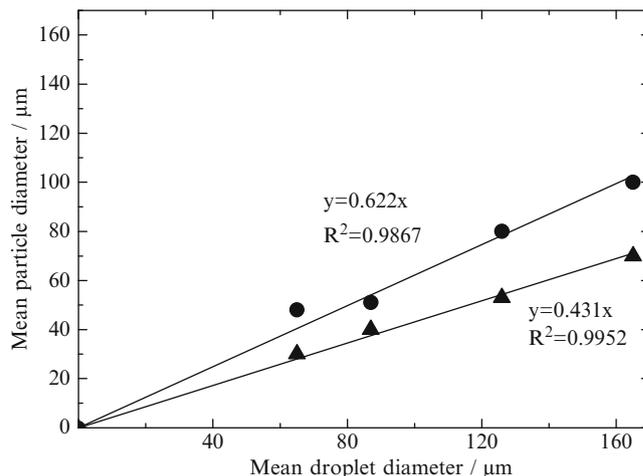
**Fig. 3** Relationship between the particle diameter in the resultant gels and the droplet diameter. Dispersed phase: sodium silicate with 6wt% SiO<sub>2</sub> in 1 M H<sub>2</sub>SO<sub>4</sub> injected at 350 Lm<sup>-2</sup> h<sup>-1</sup>. (●) Hydrogel. (▲) Xerogel
