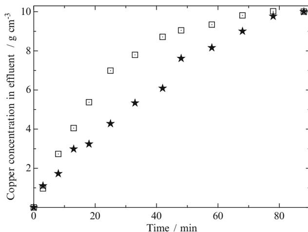
**Fig. 5** Chemisorption of  $\text{CuSO}_4$  on silica gel in a continuous flow stirred cell with slotted pore membrane. The copper concentration in influent was  $10 \text{ g cm}^{-3}$ , the flow rate of influent was  $7 \text{ ml min}^{-1}$ , and the particle loading in the cell was 2.5 g. (□) Non-treated silica gel. (★) Silica gel functionalised with 3-aminopropyltrimethoxysilane
