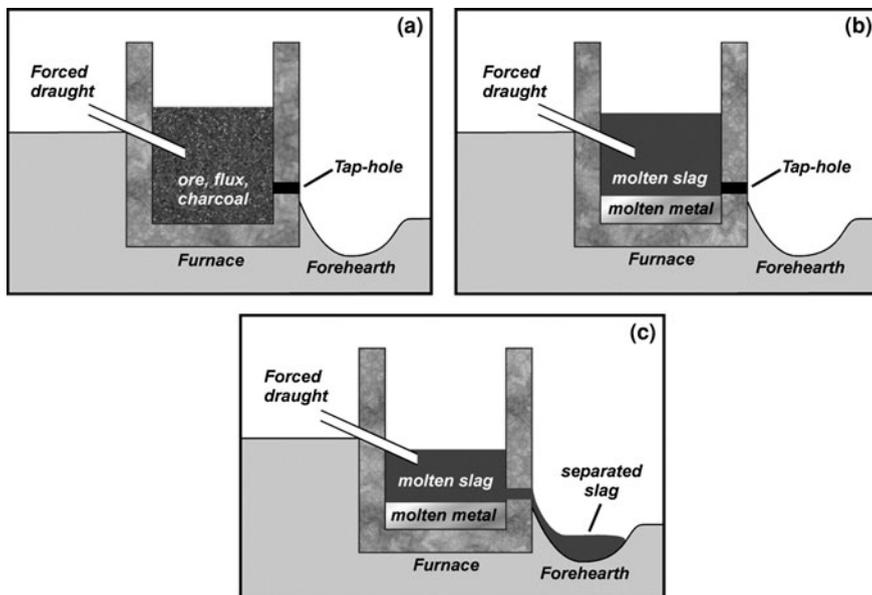
**Fig. 2.2** Smelting process: ore, flux, and charcoal are mixed in the smelting furnace and fired (a); heating produces immiscible layers of molten metal and slag (b); the tap-hole is removed, allowing the slag to drain off into the forehearth (c)
