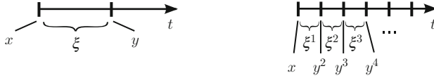
Fig. 2.1 Temporal structure of a two-stage ( left ) and a multi-stage ( right ) recourse problem. In the left time line , the wait-and-see decision y may depend on x and \xi . In the right time line , the wait-and-see decision y^s may depend on x and \xi^s , s < t
