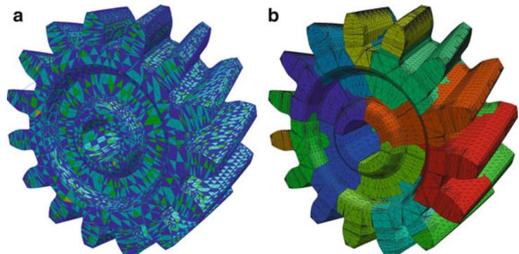
Figure 10.8: A mesh that is (a) colored based on facet connectivity such that cells that share a common facet have different colors and (b) partitioned into 12 parts, with each partition indicated by a color.
