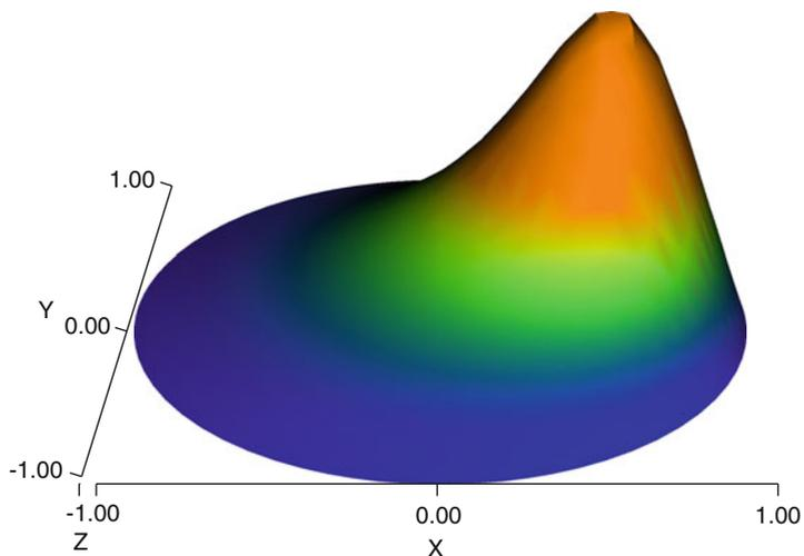
Figure 1.3: Plot of the deflection of a membrane.
