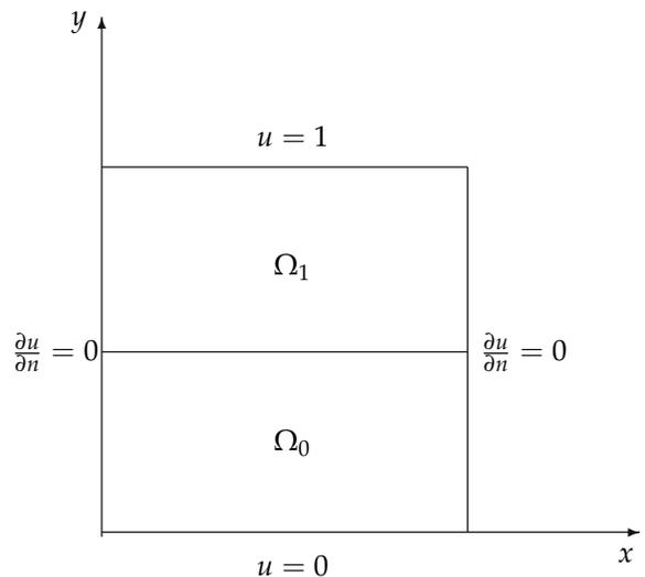
Figure 1.9: Sketch of a Poisson problem with a variable coefficient that is constant in each of the two subdomains  $\Omega_0$  and  $\Omega_1$ .
