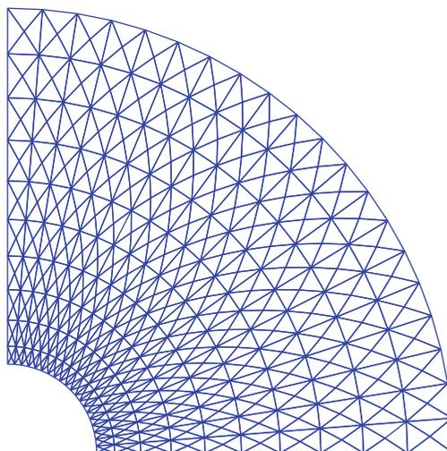
Figure 1.8: A hollow cylinder generated by mapping a rectangular mesh, stretched toward the left side.
