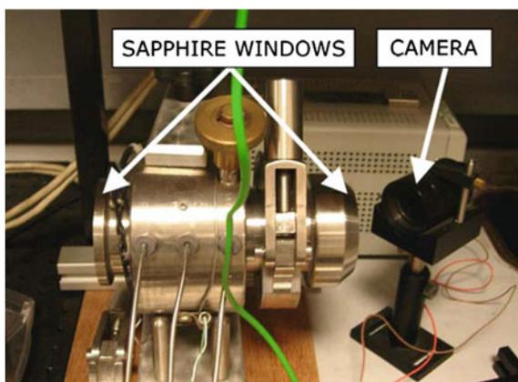
which the pressure was decreased to ambient pressure at controlled depressurization rate ( $dP/dt$ ). During this stage the temperature was either kept constant or lowered at a controlled cooling rate ( $dT/dt$ ) down to a selected temperature. At the end of the process, after a spontaneous cooling to room temperature (RT), the Teflon mould containing the foamed sample was removed from the autoclave.
