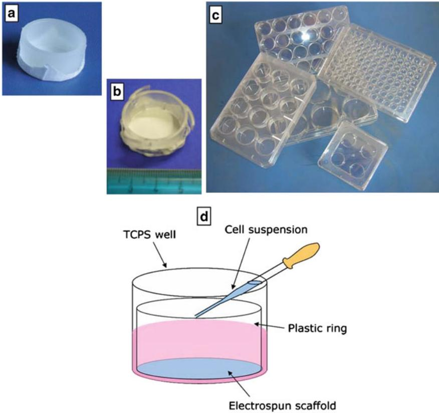
**Fig. 2.5** **a** ES scaffold fixed on a Teflon plastic ring by using medical-grade silicon, **b** ES scaffold fixed on a CellCrown<sup>TM</sup>6 plastic ring (Scaffdex), **c** common TCPS multiwell culture plates (different well dimensions are available) and **d** schematic representation of cell culture experiments: the ES sample fixed on the plastic ring is inserted into the TCPS well and cells are seeded on the upper surface of the scaffold
