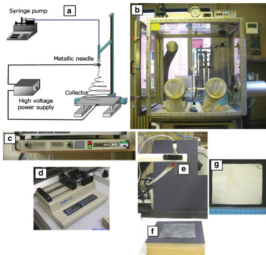
**Fig. 2.3** a Scheme of the ES process, b glove box containing the ES apparatus composed of: c high voltage power supply, d syringe pump, e metallic needle and f collector. g representative picture of ES mat deposited on aluminium plate collector ( $10 \times 10$  mm)
