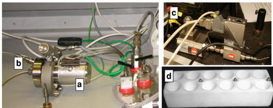
**Fig. 2.1** ScCO<sub>2</sub> foaming apparatus **a** autoclave, **b** thermocouple, **c** back pressure regulator system and **d** Teflon mould with 12 wells for batch scaffold production. This mould was designed with a detachable base to allow easy removal of scaffolds after fabrication
