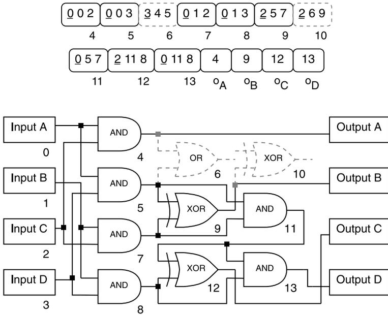
**Fig. 2.2** A CGP genotype and corresponding phenotype for a two-bit multiplier circuit. The underlined genes in the genotype encode the function of each node. The function look-up table is AND (0), AND with one input inverted (1), XOR (2) and OR (3). The addresses are shown underneath each program input and node in the genotype and phenotype. The inactive areas of the genotype and phenotype are shown in grey dashes (nodes 6 and 10).
