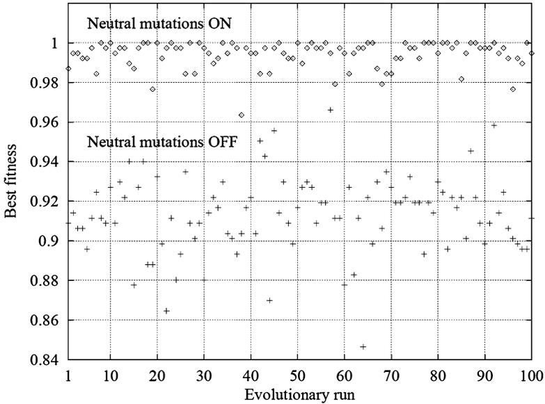
**Fig. 2.8** The normalized best fitness value achieved in two sets of 100 independent evolutionary runs of 10 million generations. The target of evolution was to evolve a correct three-bit digital parallel multiplier. In one set of runs, neutral drift was allowed, and in the other, neutral drift was not allowed. The evolutionary algorithm was unable to produce a correct circuit in the second case.
