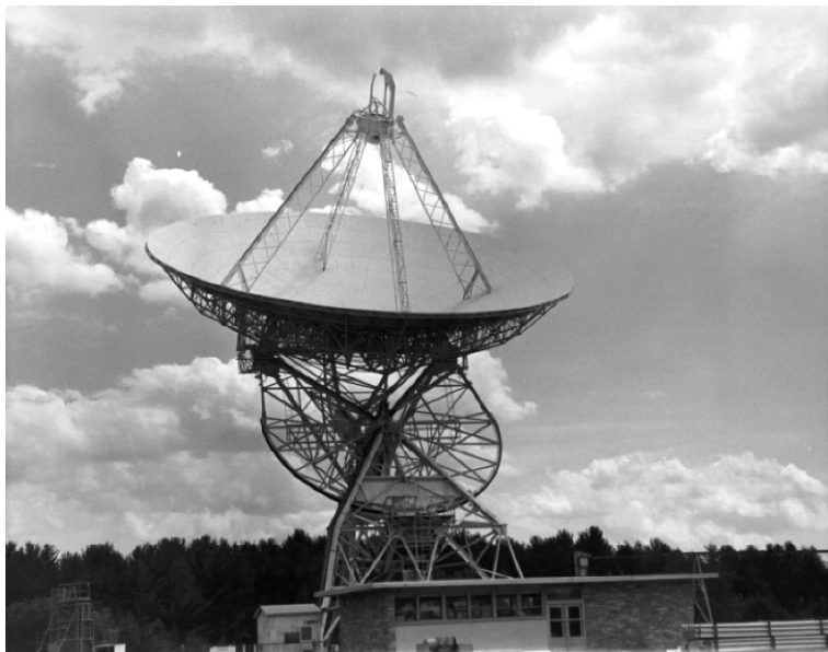
Fig. 2.1 The 85-foot diameter Howard Tatel Telescope at the National Radio Astronomy Observatory, Green Bank WV, used by Frank Drake for his Project Ozma observations in April and May of 1960.
