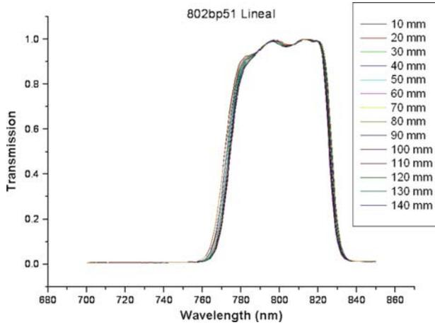
Fig. 4 Transmission of one of the order sorter filters versus wavelength for different areas of the filter showing the excellent uniformity of the response
