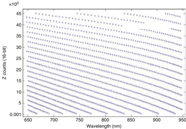
Fig. 5 Red TF calibration: Etalon gap in counts of 16-bit versus wavelength. Each set of points defining a straight line represent a different order. For each wavelength the different orders define the different FWHMs that can be tuned at this wavelength
