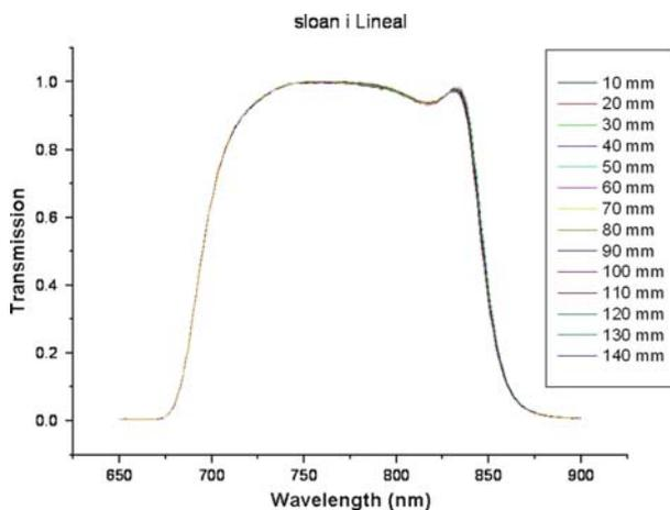
Fig. 3 Transmission of the  $i'$  filter versus wavelength for different areas of the filter showing the excellent uniformity of the response
