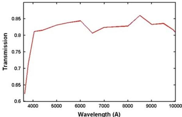
**Fig. 2** OSIRIS transmission versus wavelength. Includes all OSIRIS optics but does not include telescope, detector or filters/grisms
