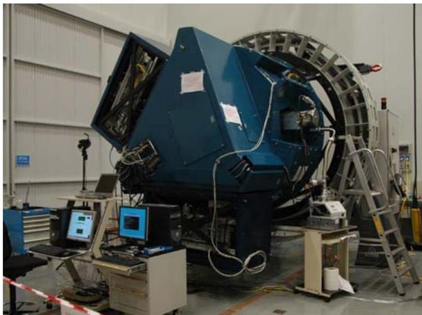
**Fig. 1** OSIRIS instrument mounted at the Nasmyth rotator of the AIV room at the IAC for laboratory tests
