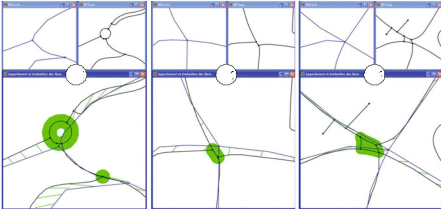
**Fig. 2.1.** Data matching results. In each of the three subfigures, the less detailed network (*top left*), the most detailed one (*top right*), and their superimposition and matching (*bottom*) are represented
