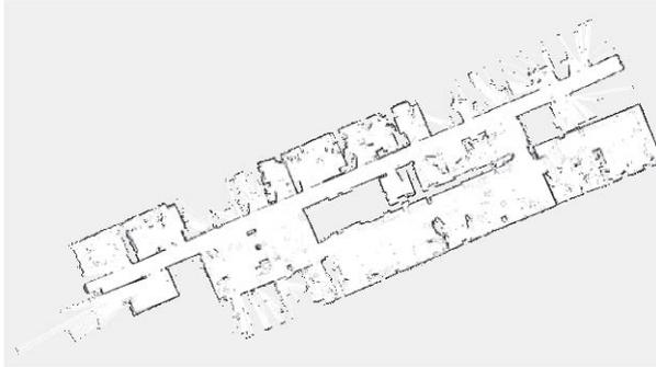
Figure 2.3: An occupancy grid representation. The cells' likelihood of being occupied is represented by their gray values, ranging from white (unoccupied) to black (occupied)
