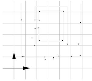
Figure 2.5: Landmark-based representation consisting of point landmarks referenced in a global coordinate system
