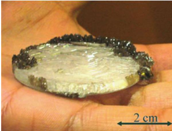
**Fig. 11.3** A 2-inch GaN crystal grown by the Na-flux LPE method. About 0.5 at% C had been used as additive to reduce the parasitic nucleation of GaN [12] (Reprinted with permission. © 2008, Elsevier Publishers.)
