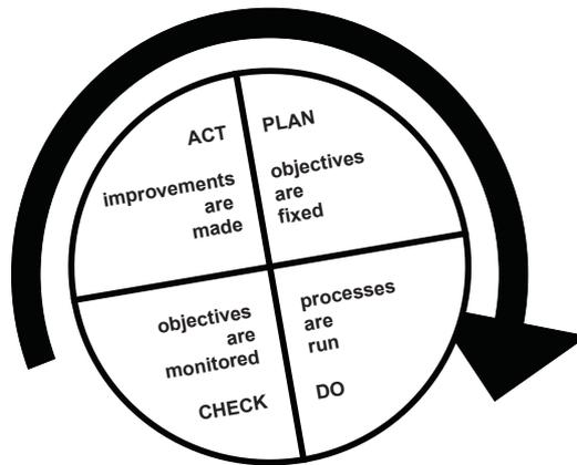
Fig. 2.7. The Deming wheel for quality control.
