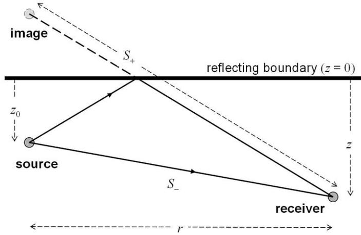
**Figure 2.3.** Radiation from a point source in the presence of a reflecting boundary.
