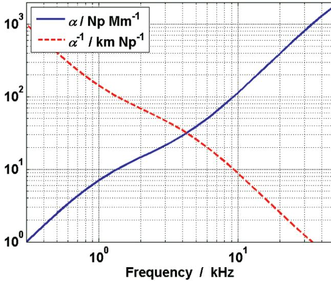
**Figure 2.1.** Numerical value of attenuation coefficient *vs.* frequency of sound in seawater  $\alpha$  (expressed in units of nepers per megameter) and of its reciprocal,  $\alpha^{-1}$  (in kilometers per neper), calculated using Equation (2.2) for the specified representative conditions:  $S = 35$ ;  $T = 10^\circ\text{C}$ ;  $z = 0$ .
