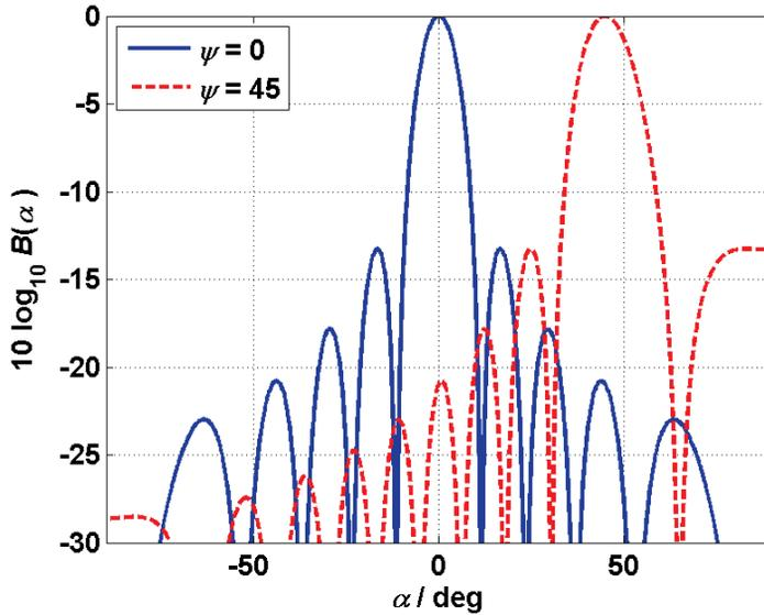
Figure 2.5. Beam patterns for  $L/\lambda = 5$  and steering angles 0, 45 deg as indicated.
