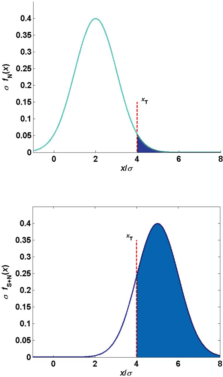
**Figure 2.6.** Probability density functions of noise (*upper graph*) and signal-plus-noise (*lower*) observables. The threshold for declaring a detection,  $x_T$ , is shown as a vertical dashed line. The shaded areas are the probabilities of false alarm (*upper graph*) and detection (*lower*). The example shown is for the case  $\bar{x}_N = 2\sigma$ ,  $\bar{x}_{S+N} = 5\sigma$ , and  $x_T = 4\sigma$ .
