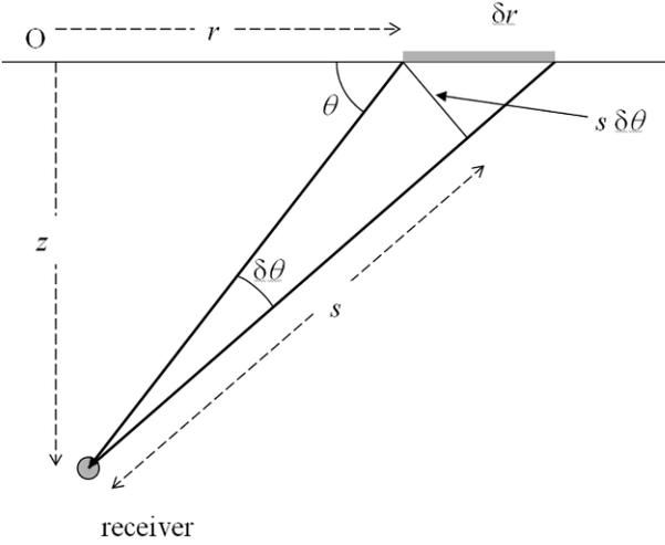
**Figure 2.4.** Radiation from a sheet source element of width  $\delta r$ .
