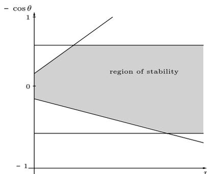
**Fig. 15.** Stable contact angles for Wenzel type drops
