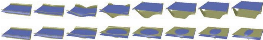
**Fig. 12.** Each row shows on the periodic cell a family of coating surfaces together with the liquid vapor interfaces of the corresponding vapor inclusions in the wetting regime of the Cassie–Baxter model. In the *first row* the transition in the surface configuration from a wavelike pattern in one axial direction to more spike type structures is depicted *from left to right*, whereas in the *second row* the transition from the same wave pattern to elongated troughs is shown
