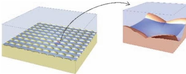
**Fig. 11.** The effective contact angle on a rough surface is calculated based on the numerical solution of a free boundary problem on a fundamental cell. The liquid vapor interface of the vapor inclusion on the surface forms a minimal surface with a contact angle on the surface of the solid determined by Young’s law
