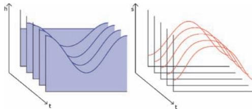
**Fig. 2.** Evolution of a coating with a marangoni flow introduced by an inhomogeneous solvent concentration
