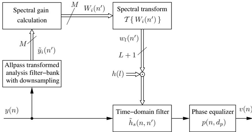
Fig. 2.16. Allpass transformed FBE for adaptive subband filtering.
