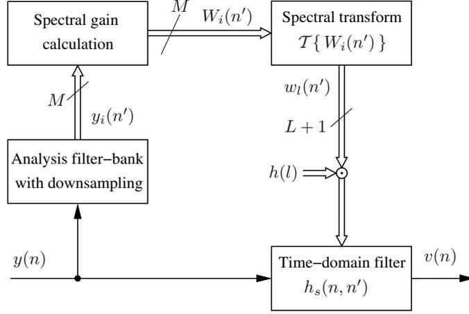
**Fig. 2.11.** Filter-bank equalizer (FBE) for adaptive subband filtering.
