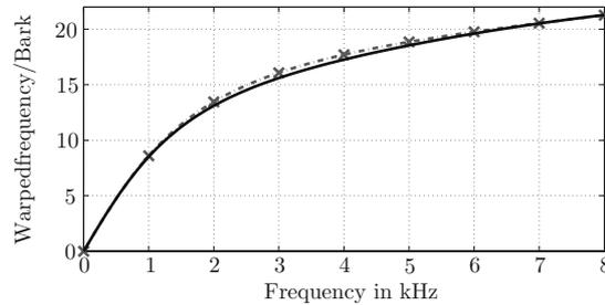
**Fig. 2.6.** Approximation of the Bark frequency scale: The solid line corresponds to the analytical expression of Eq. 2.21. The dashed line marks the frequency warping for an allpass transformation with  $a = 0.576$  and a sampling frequency of 16 kHz.
