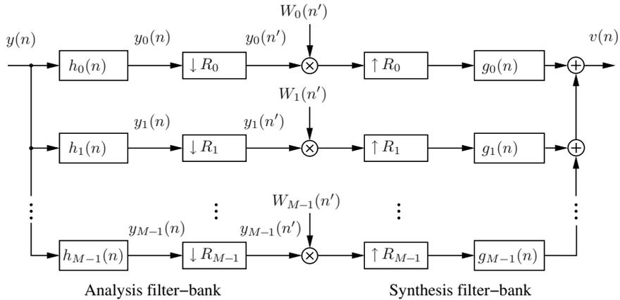
**Fig. 2.1.**  $M$ -channel analysis-synthesis filter-bank (AS FB) with subsampling and spectral weighting.
