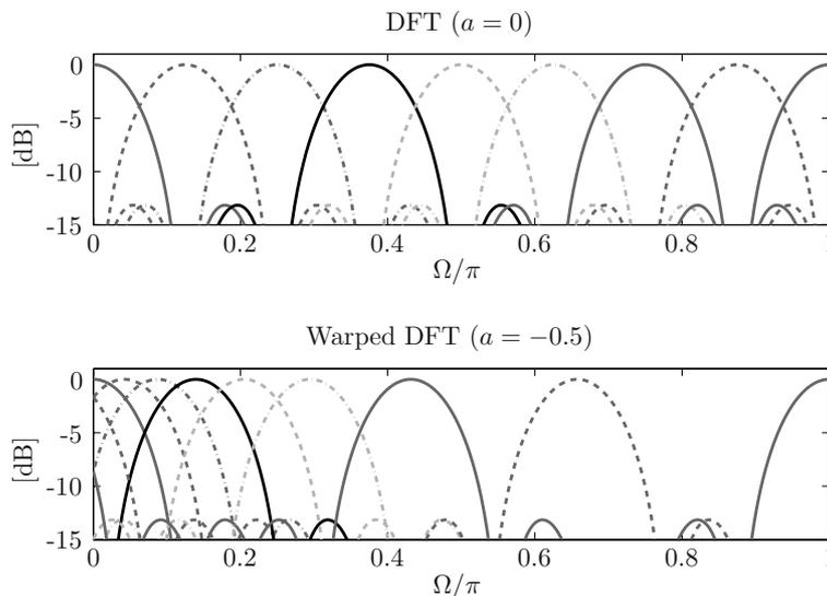
**Fig. 2.9.** Magnitude responses of the subband filters for a DFT and warped DFT with  $M = 16$  channels.
