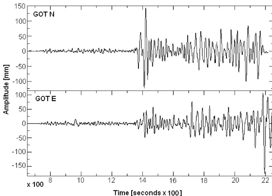
**Fig. 1.4.** Seismograms of the 1906 San Francisco earthquake recorded in Göttingen, Germany, some 9100 miles away from the earthquake source; (top) NS components, (bottom) EW component (from Wald et al. 1993).
