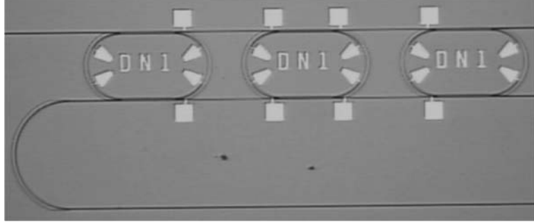
Fig. 2.15. Photograph of a parallel coupled triple ring resonator
