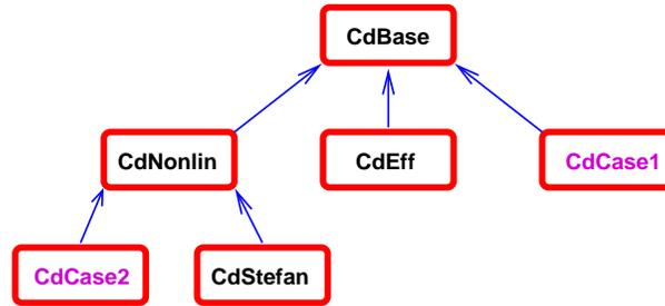
**Fig. 6.1.** A sketch of the convection-diffusion solver, with the base class `CdBase`, the efficient implementation `CdEff`, the more general nonlinear convection-diffusion solver `CdNonlin`, and the specialization `CdStefan` of `CdNonlin` to solve problems with freezing or melting. The classes `CdCase1` and `CdCase2` just indicate possible user-defined small classes that customize the  $b$ ,  $k$ , and  $f$  functions in a particular problem. The arrows indicate class derivation.
