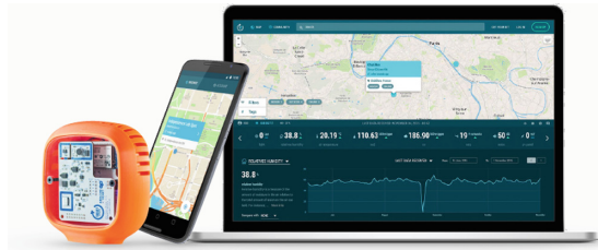
Fig. 1. The Smart Citizen kit, mobile app and data visualization platform.
